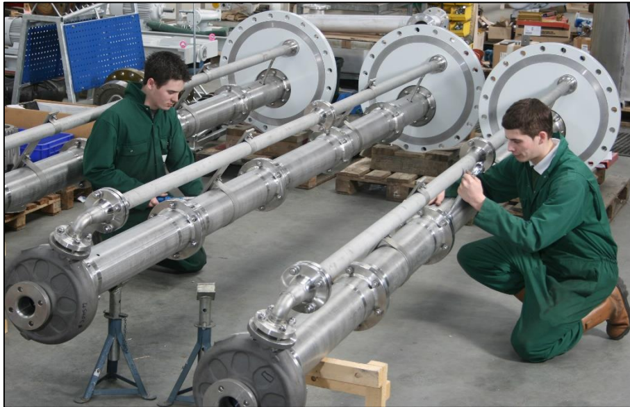
Amarinth engineers undertaking final assembly of pumps
