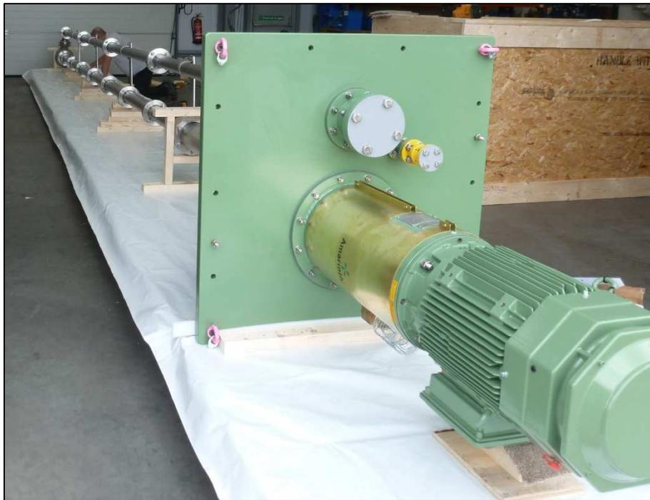
Amarinth 9.5m long API 610 VS4 vertical sump pump being packed ready for shipping to the Borouge petrochemicals complex in Ruwais, Abu Dhabi
