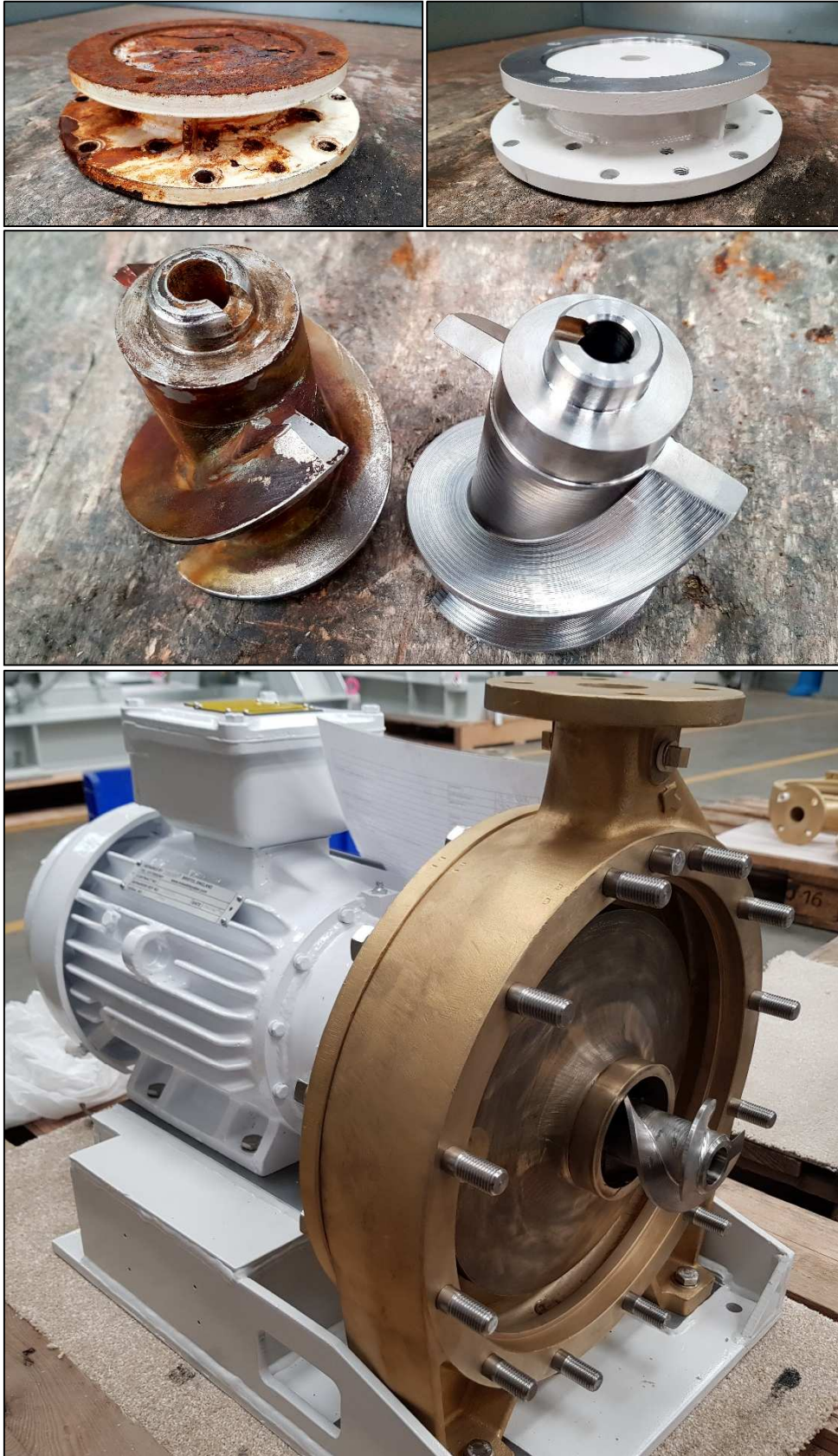
Comprehensive refurbishment by Amarith of third-party OEM pump
