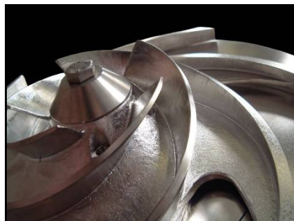
Scalloped and electro-polished impeller
