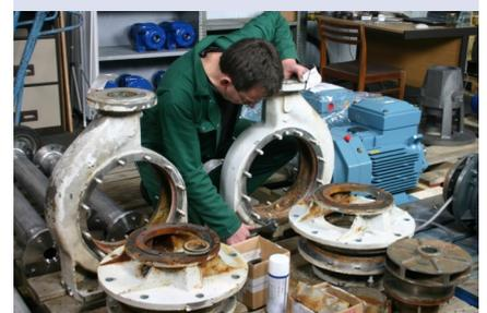
**Amarinth decontaminated the pumps and refurbished them with bearing isolators and new mechanical seals in order to make them ATEX compliant.**
