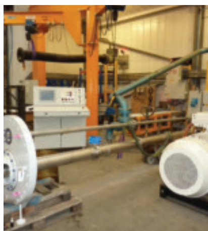
Figure 3. The rig had to be suitable for use with pumps having to drive motors ranging from just a few kW up to more than 300 kW.
