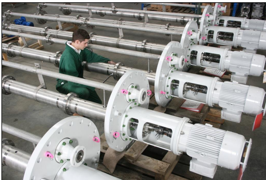
Amarinth API 610 VS4 Pumps during assembly
