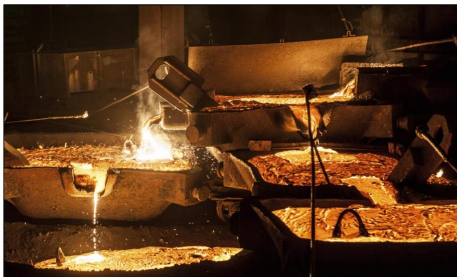
Pouring liquid titanium from the arc furnace
