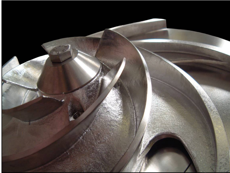
Scalloped and electro-polished impeller
