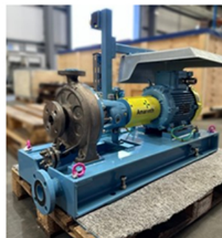
Amarinth pump nearing the end of assembly
