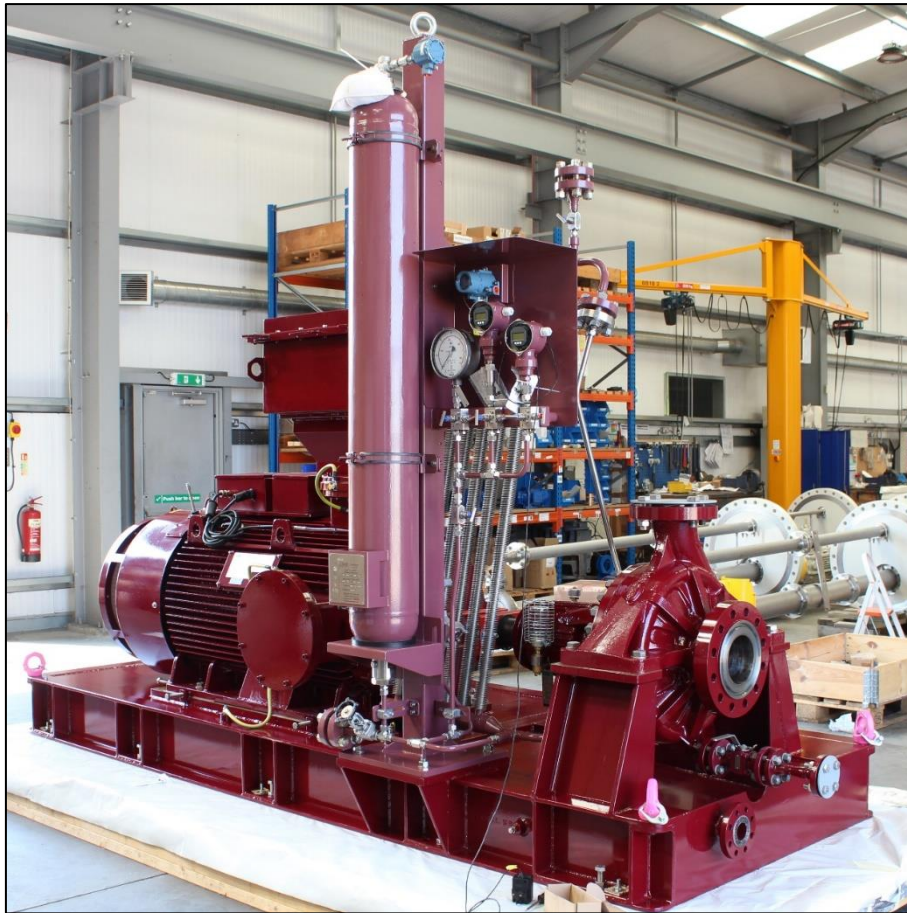
Amarinth API 610 OH2 pump being readied for delivery to the ADNOC Bu Haseer full field development project
